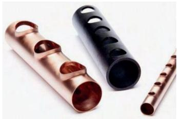
WinterTech produces tube headers, also known as manifolds, for use in a variety of heat exchanger applications. Tube holes can also be T-Drilled (collared), drilled, or punched per requested requirement.
