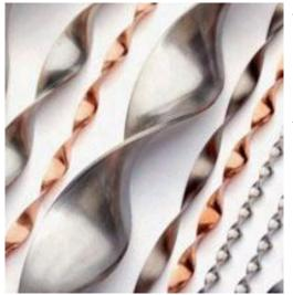
The twisted style turbulators offer a large range of size and length to fit any application. Turbulators are inserted into heat exchanger tubing to increase the turbulent flow through a tube, efectively increasing heat exchange rates and abilities. Turbulators act to mix the fluid or gas on the inside of the tube.
