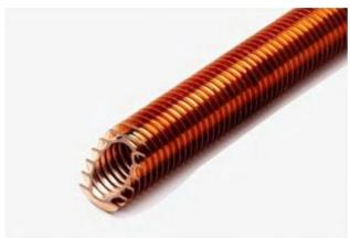
The WinterTech Medium-High Finned Tube is made from mono extruded copper alloys. The WinterTech-M height is within 0.140" (3.5mm). Extruded fin tube are formed helically out of a mono-metal tube.
