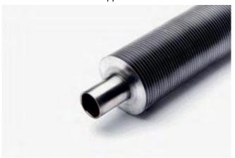
WinterTech embedded finned tubing offers exceptional thermal efficiency at higher temperature ranges with solid fin-to-tube contact. Fins are mechanically locked into a helical groove in the outside of the tube.
