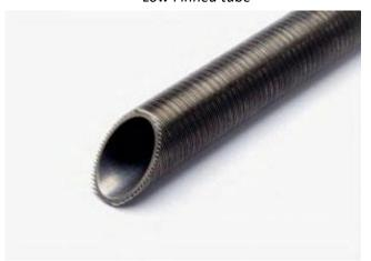
WinterTech Low Fin (Integral) tubing is a type of extruded tubing that consist of shorrt low fins. The low fins. The low fin tube has the adventage of adding surfce area to a smooth tube while maintaining the same outside diameter.
